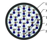
LSOH (SHF1) Outer Sheath XLPE Insulation Tinned Copper Drain Wire
